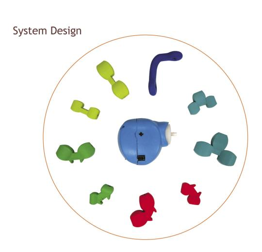
The Topobo system is comprised of ten primitives that are connected with Lego Technics® connectors. Nine of these primitives are called "Passive" because they form static connections. One motorized "Active" forms dynamic connections which allows the system to reproduce manipulations to a structure.
