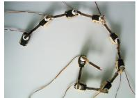
A Queen does not need to be mechanically attached to the creation it is programming, so it can also be used as a remote controller. Remote programming with a Queen gives a child synchronous input and output feedback during programming, allowing the child to observe their creation's motion while they are composing it.
