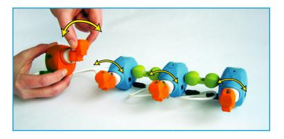
Programming with a Queen: In both record and playback modes, all motions of the Queen are imparted directly to all Actives connected to the Queen.
