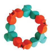
Topobo has 12-fold symmetry and can support free form or patterned building. Green Tetras can be connected flat into a pentagon (above), or notched together into a tetrahedral (right).
