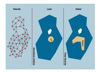
Proto decomposes selfmanaging systems into Discrete, Local and Global abstraction layers. This allows high level specification of distributed behaviors.
