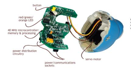
Custom electronics handles memory, processing, communications and power distribution.
