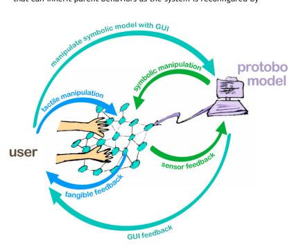
Cooperative interaction with a kinetic material: the kinetic material's behavior is affected by a combination of the user's tactile input and the Protobo symbolic model. The user will manipulate both the Proto program, via a GUI, and the kinetic material, via tactile gestures.
