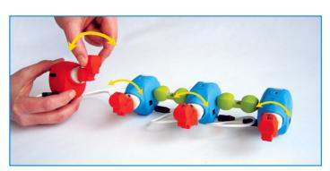
Special orange actives called Queens can control many other Actives. In both record and playback, all motions made to a queen are mimicked by the other actives connected to the Queen.
