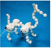
Second generation parts were modeled with 3D CAD software and 3D printed in ABS plastic. This allowed us to house the electronics and motor in a single case. Parts were later mass produced based on this design.
